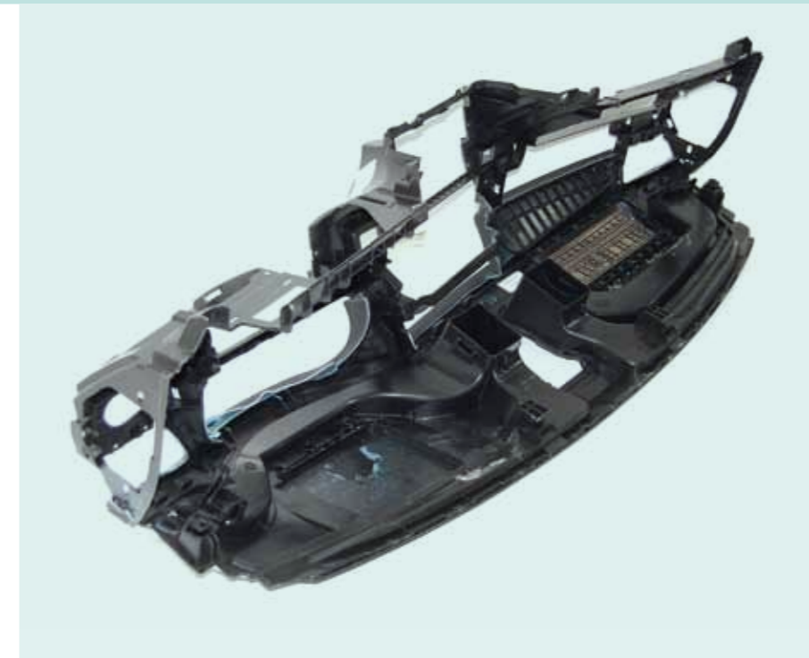
The foamed instrument panel of the new BMW 7 offers a weight reduction of 2.82 kg compared to the old BMW 7
