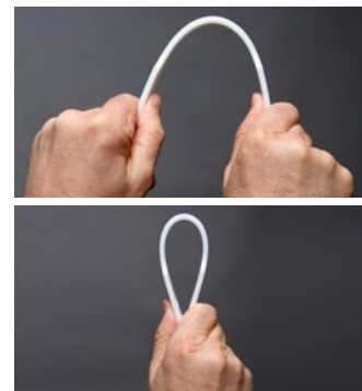
Conventional TPU impact modified POM
