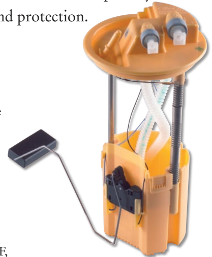
Siemens VDO uses the new Hostaform® grade EC140XF in the fuel system of the Ford Transit. The special modification of the polyacetal ensures good electrostatic charge dissipation.
